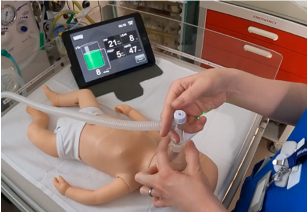
Fig. 2 – Monivent NeoTraining in use during the training intervention. The visual display during optimal ventilation is depicted here. All data from the sensor module is transmitted wirelessly to the external monitor which displays continuous feedback of ventilation parameters.
